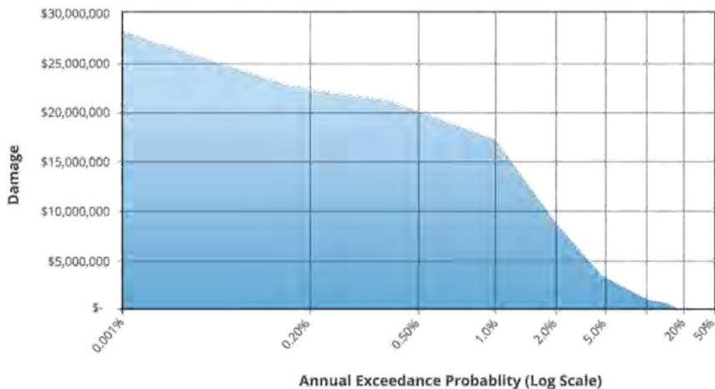
Figure 29 A Sample of a flood damage curve for a range of AEP events (ARR 2019)
