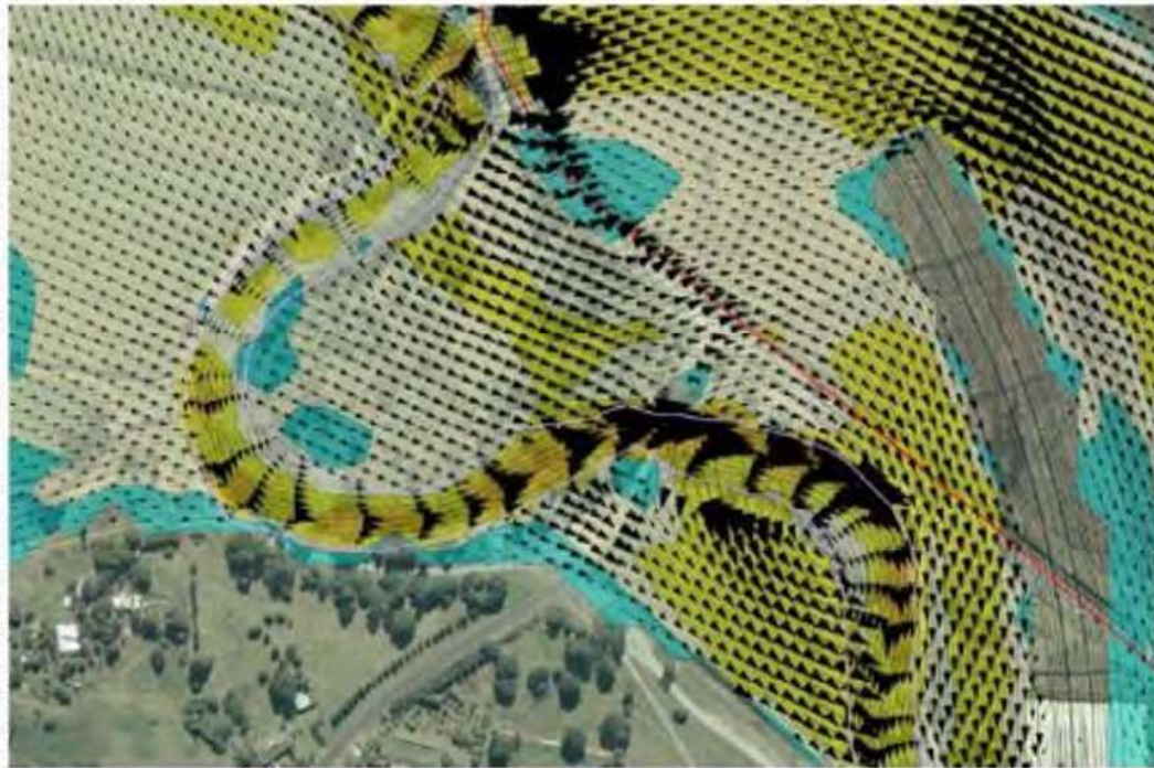
Figure 12 1D/2D Hydraulic Model results showing flow patterns
