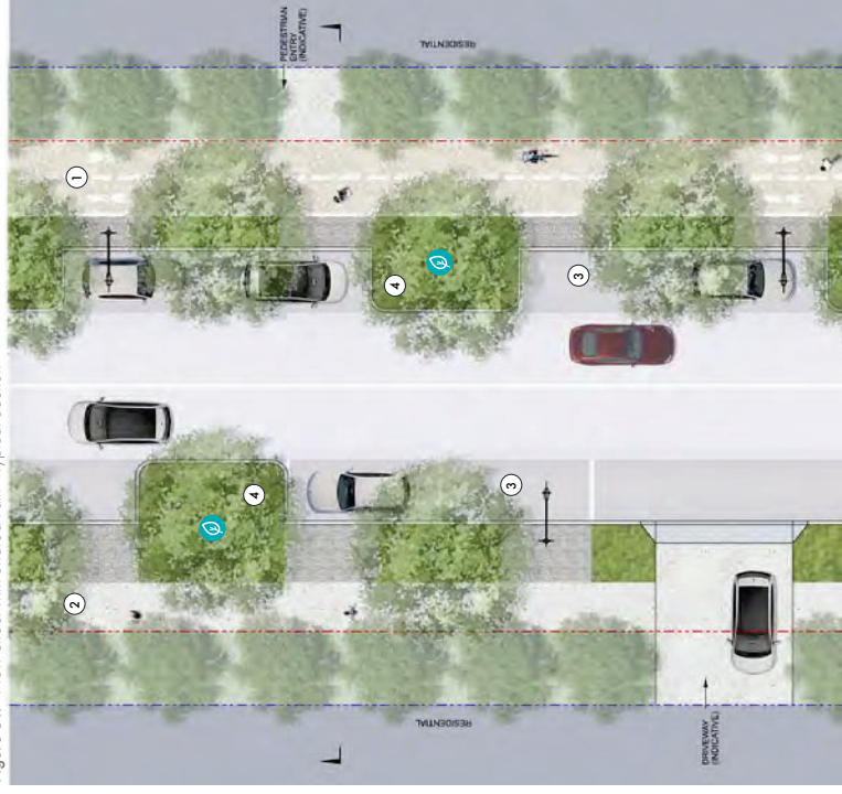
Figure 61. New Street with Shared Path - Typical Section
