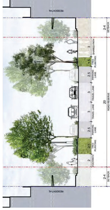
Figure 61. New Street with Shared Path - Typical Section
