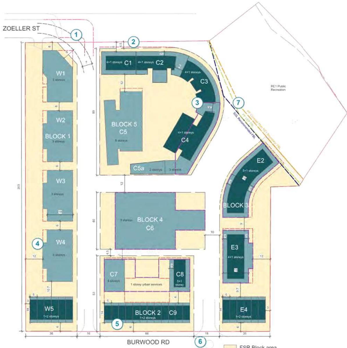
Figure 72 Recommended site layout prepared by Studio GL with building envelopes used to calculate FSR
