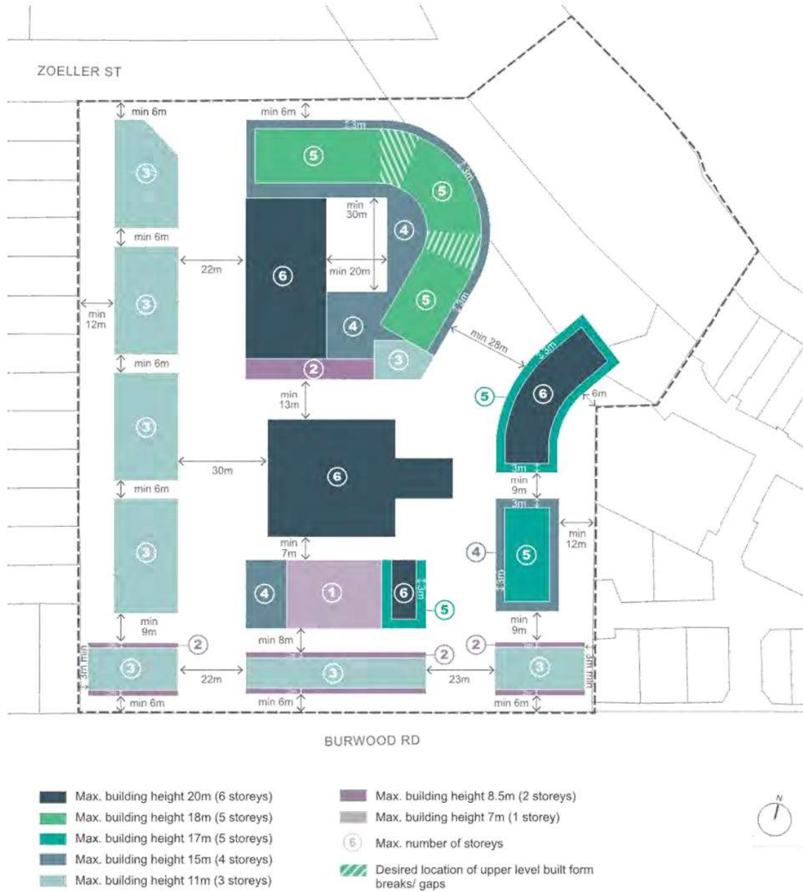
Figure K19-7 Building Envelope Controls Plan
