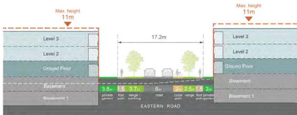
Figure K19-14 Section 6: Local street section
