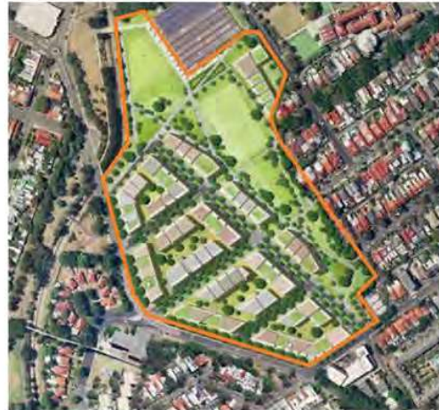
Figure 33 Example of a Precinct Plan showing new roads and through site links which connect to the surrounding neighbourhood (source: NSW DPE 2015, p.25)
