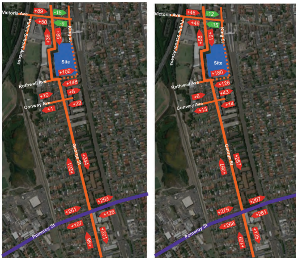
Figure 5-7 Estimated total future traffic increase - 2036 AM (left), 2036 PM (right) 1-hour peak link flows
