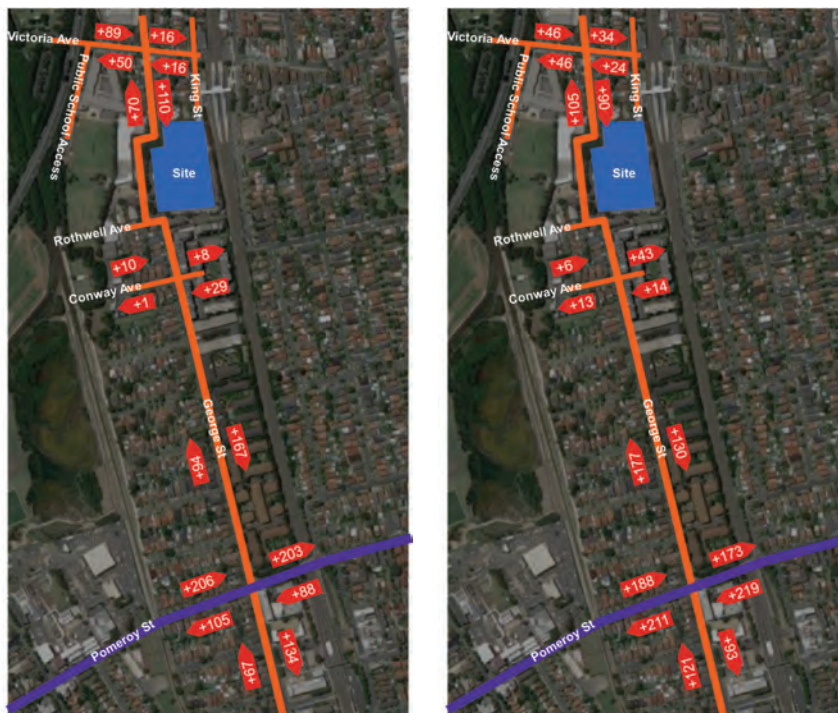
Figure 5-6 Estimated background traffic increase – 2036 AM (left), 2036 PM (right) 1-hour peak link flows
