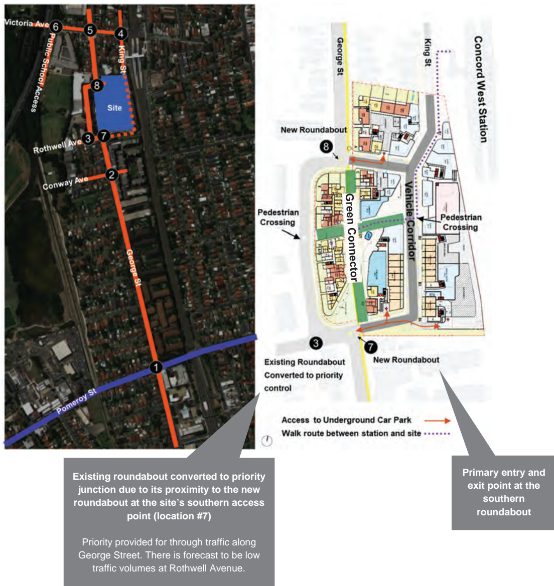
Figure 6-1 Site access to underground car park, new intersections and walking route between station and site
