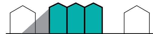
The greatest limitation for complying terraces is the potential overshadowing impacts on neighbours
