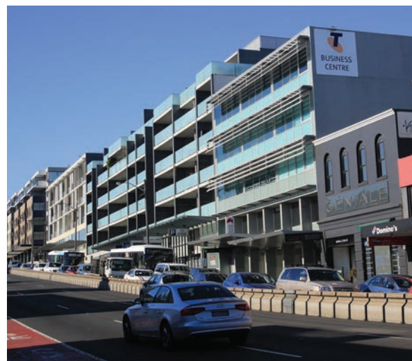
A five storey street wall height is perceived as a higher street wall height due to topography and building articulation
