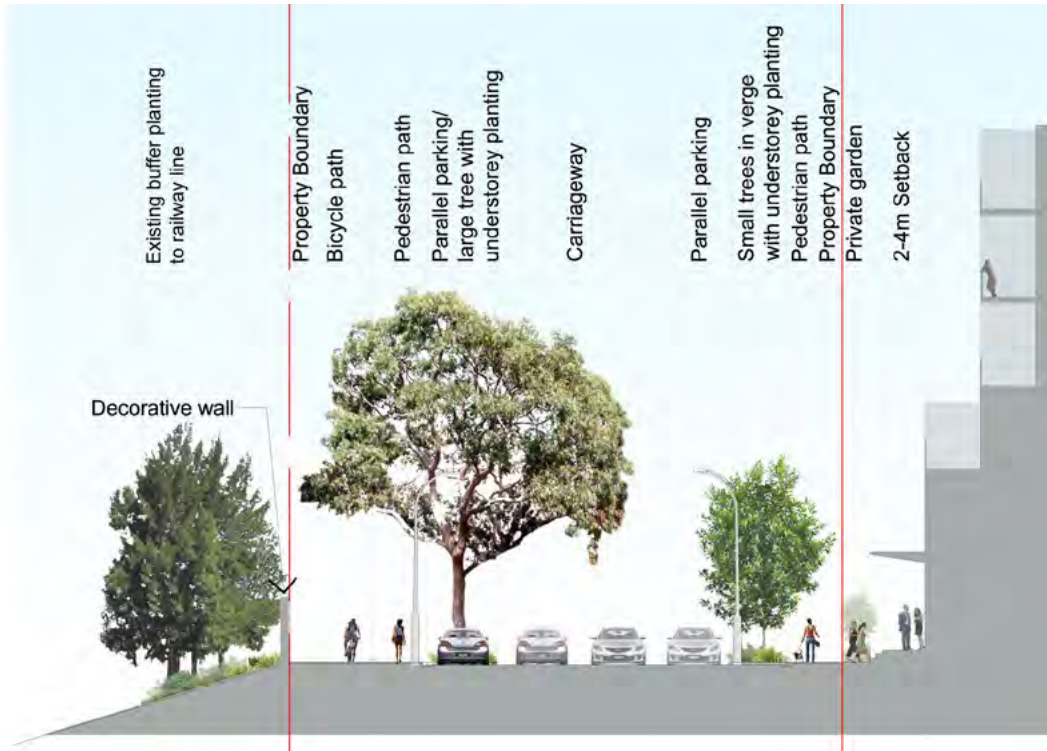
Figure K16-11 Street section - Commuter Street
