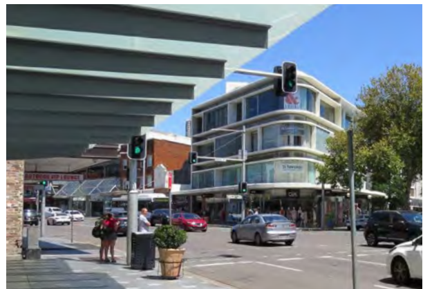
Translucent awnings allow for more daylight access to the footpath and shopfronts
