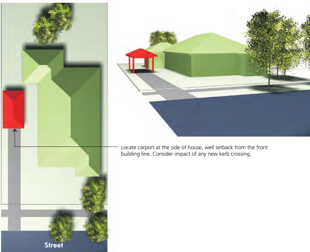
Figure B3.2 Location of car parking at the side behind the front alignment
