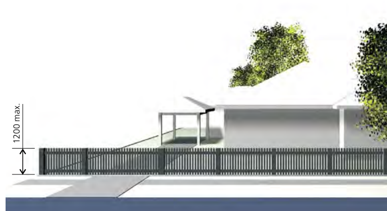
Figure F5.2 Example of open front fencing with a height of 1200mm
