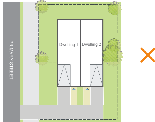
Figure E4.5 Undesired development - dwellings not orientated towards the street frontage
