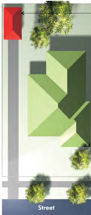
Figure B3.4 Location of car parking at the rear of the site with access from street frontage
