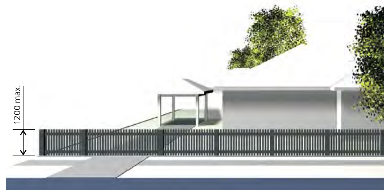
Figure E4.14 Example of open front fencing with a height of 1200mm
