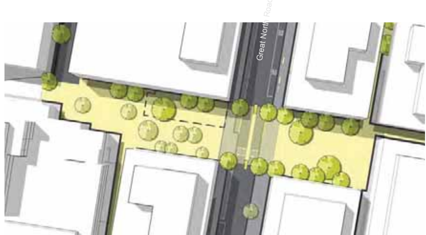
Figure 9. Shadows 21 March (Autumn) at 2pm - Fred Kelly Place (extended) and the new town square
