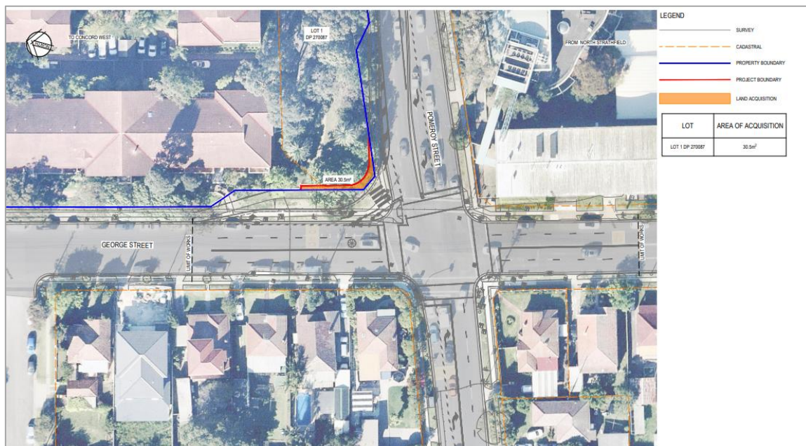
Figure 33: Land Acquisition to deliver alternative Council George/Pomeroy intersection design (Source: Council mapping)
