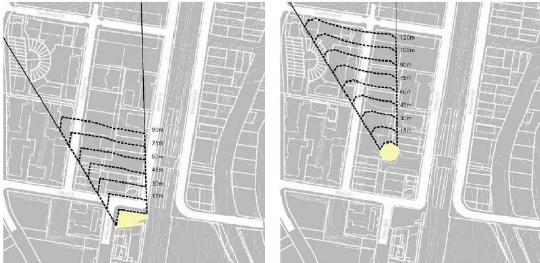
Figure 8: Solar Access Planes (defining potential heights of buildings in relation to areas where solar access must be either fully protected, i.e. Town Square, or maximised i.e. child care centre, mid-block plaza and laneways).
