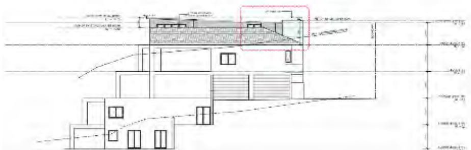
West elevation with extended lift shaft shown in green and connecting corridor behind, both of which will be visible in the streetscape
