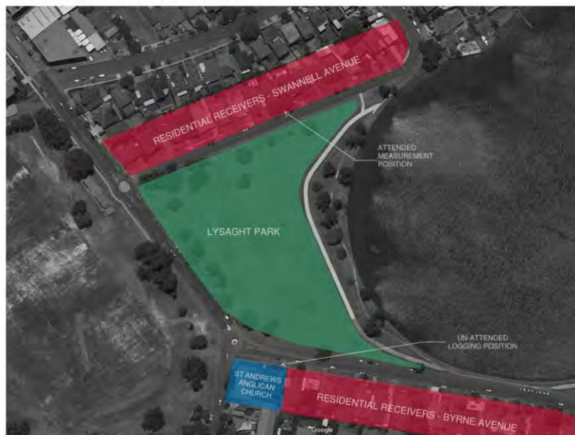
Figure 1: Site and noise monitoring locations
