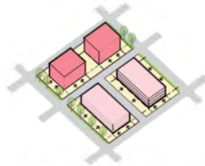
1. Provide landscape setback in residential zone of 5m and 8m along priority green streets.
