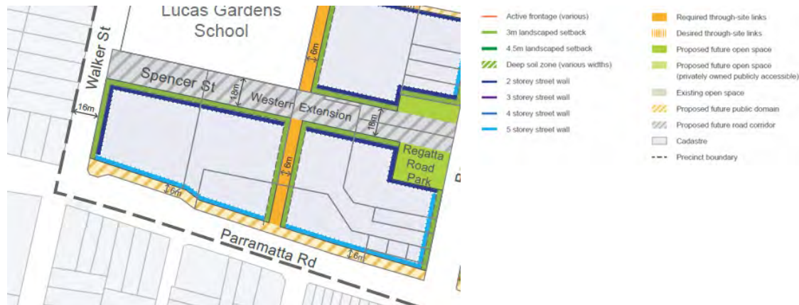
Figure 7 Draft DCP – Street wall provisions
