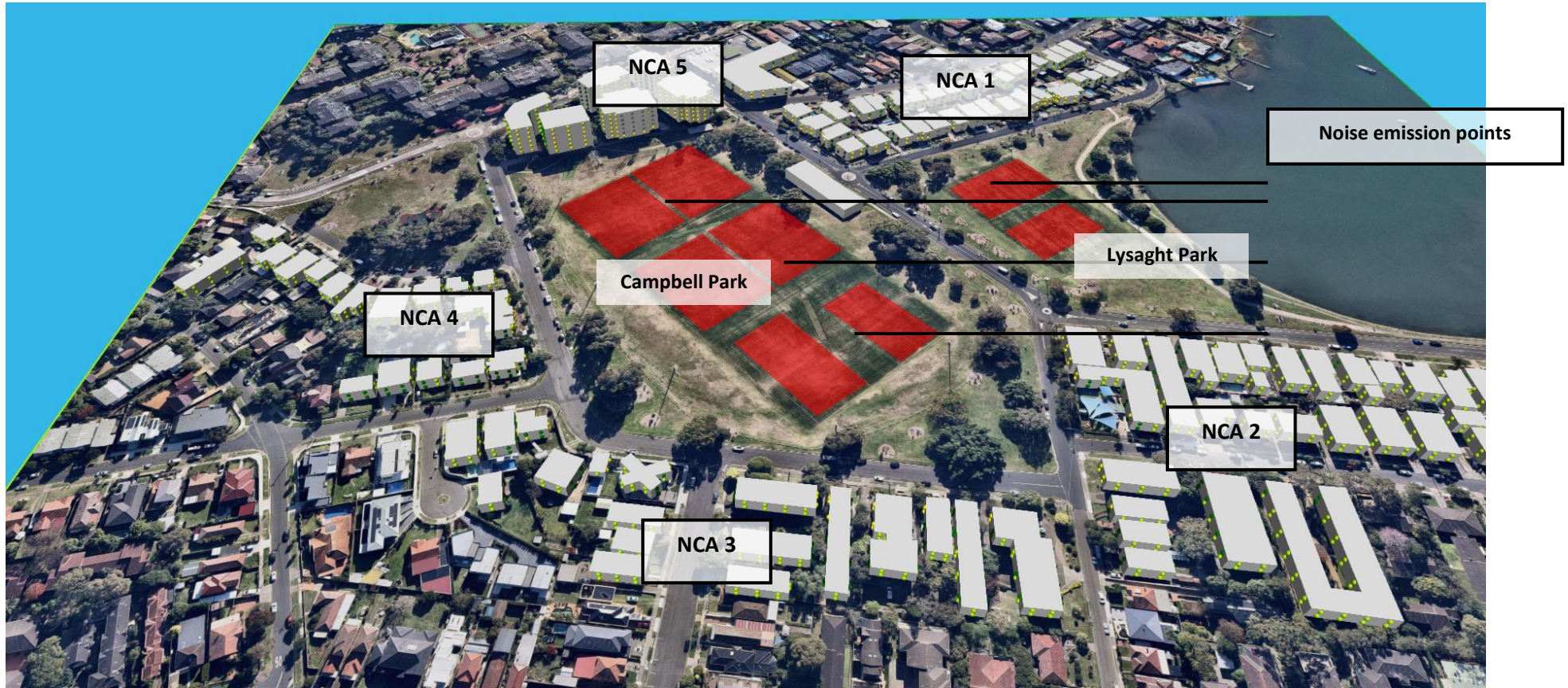
Figure 5-1 Scenario 1 – 3D View of Assumed Noise Emission Points for 8 Youth Teams Practise Matches
